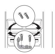
7. Unscrew the retaining screw for the self-closing mechanism on the bottom of the fridge compartment door.
